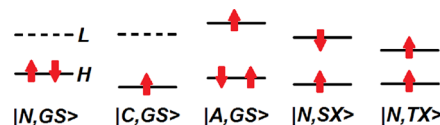
Figure 1. Main electronic states for a two-orbital site occupied by one, two, or three electrons. H and L stand HOMO and LUMO orbitals, respectively. The latter is represented by a dashed line when it is unoccupied or “virtual”. The orbital energies depend on the state to indicate that our model goes beyond the independent particle picture by including electron–electron interactions.
